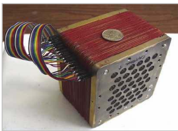
Stack DMFC 80 W (30 celle, 45 cm²) - LANL
